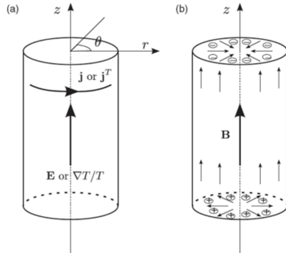
FIG. 1. Electric and thermal response of topological insulators, and thermal response of topological triplet superconductors, in a cylindrical geometry. (a) Electric ( $\mathbf{j}$ ) or thermal ( $\mathbf{j}^T$ ) current driven by applied electric field ( $\mathbf{E}$ ) or thermal gradient ( $\nabla T/T$ ). (b) A response dual to (a) where an applied magnetic field in the  $z$  direction induces charge polarization.
